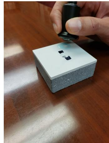
Photo 2: Ultrasonic Film Thickness Measurement
