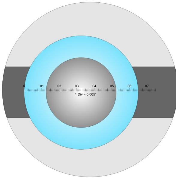
Coating film thickness is measured using a magnifier with a measuring reticle (Figure 5). In Figure 6, we are using a 7x loupe with a reticle capable of measuring  $\frac{3}{4}$  of an inch in .005" divisions (5 mils per hash mark). Note that when the measuring loupe is placed on top of the drilled hole, it is possible to measure the
