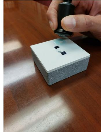
Photo 2: Ultrasonic Film Thickness Measurement
