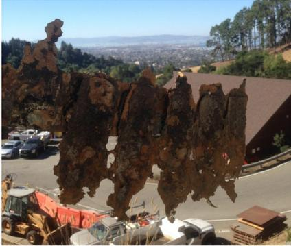
Corrosion in corrugated metal drainage pipes can often lead to structural deterioration and eventual collapse. Many owners are solving this problem by cement mortar lining drainage pipes before corrosion becomes detrimental. H&R Plumbing recently performed an application of Mainstay ML-72 Restoration Mortar on 50' of corrugated metal culvert using Madewell's horizontal mortar spinner.
