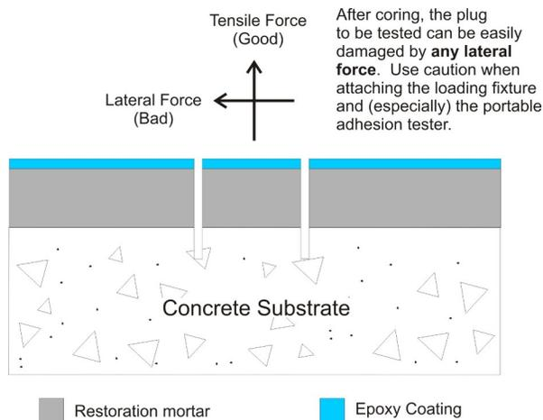
Figure 3: Schematic of Failure Modes (ASTM C 1583)
