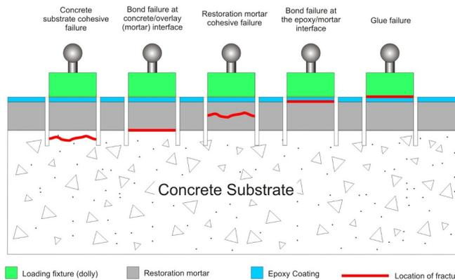
The International Concrete Restoration Institute (ICRI) Guideline No. 320-2R recognizes ASTM C 1583 as an important quality control test for bond strength of overlay materials and recommends a minimum requirement of 250 psi (1.71 Mpa). However, the guideline acknowledges that some specifiers use an acceptance criteria less than this.
