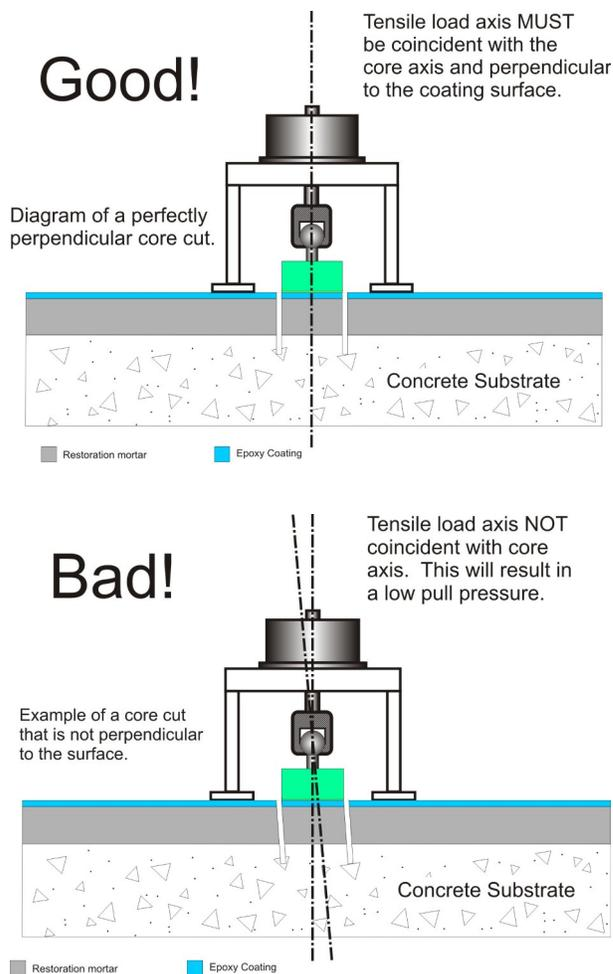
Coring the pulloff location is complicated significantly when the surface to be tested is curved (for example, on the interior walls of a manhole). Interesting fact, both ASTM D 4541 and ASTM D 7234 require that the “test area must be a flat surface large enough to accommodate the specified number of replicate tests.. ASTM C 1583 does not mention the word “flat”.
